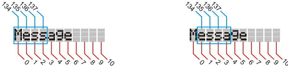
Figure 1-21: Shifting Text Through Window, Steps 3 and 4
