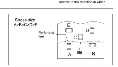
to varistor placement, consider the board breaking method as well.
