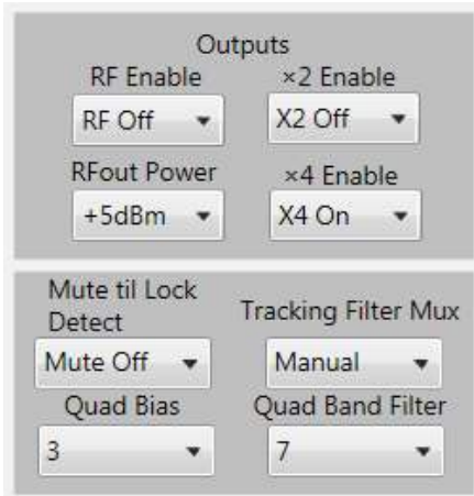
Figure 6. Recommended Quadrupler Filter Settings, 16 GHz to 18 GHz
