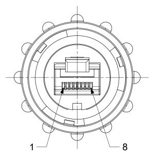
**RJ-45 FACE VIEW** (BAYONET COUPLING) SCALE: 2X
