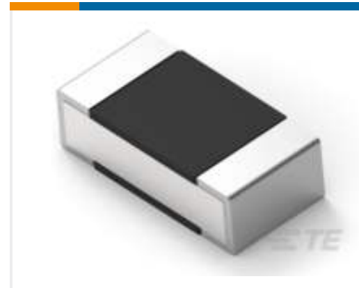
TE Part #9-2176304-8 RP 1E 0.1W 102R 0.1% 25PPM 5K RL
