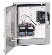
2-speed 3-phase motor starter Size 1 Two separate windings Constant or variable torque Solid-state overload relays Low SPD OLR range 0.25-1A High SPD OLR range 0.75-3.4A 110V 50HZ / 120V 60HZ coil Combination type 3Amp circuit breaker Enclosure NEMA type 1 Indoor general purpose use
