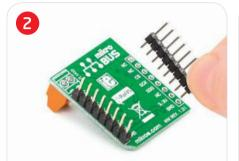
Turn the board upside down so that bottom side is facing you upwards. Place shorter parts of the header pins in both soldering pad locations.
