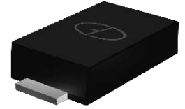
Package: eSGA (SOD-123FL)
