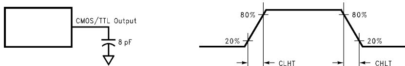
Figure 6. DS90CF384A/DS90CF364A (Receiver) CMOS/TTL Output Load and Transition Times
