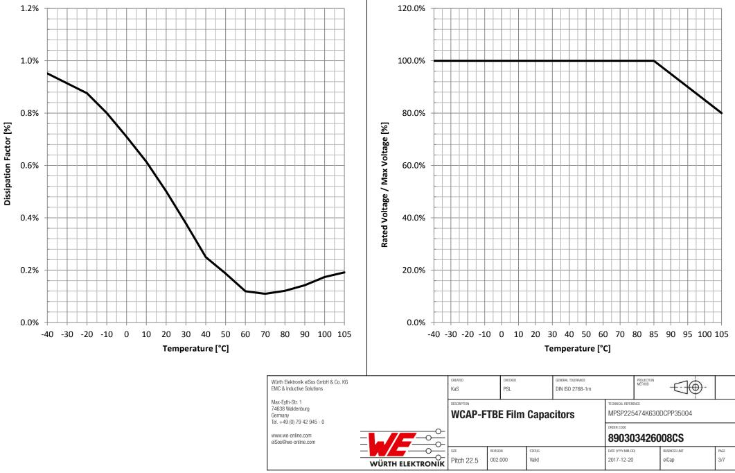
**Rated Voltage vs. Temperature:**
