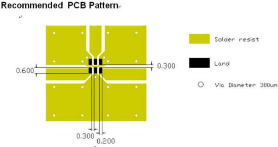
Line width should be designed to match  $50\Omega$  characteristic impedance, depending on PCB material and thickness.
