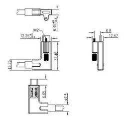
This cable includes a 10K pullup resistor between the 'CC' line and ' $V_{BUS}$ '. For systems compliant with the USB Type-C Cable and Connector Specification, the cable current will be restricted to 3.0A.
