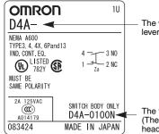
The whole switch model without lever is printed.
