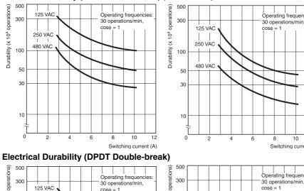
Electrical Durability (SPDT Double-break) (Ambient temperature: +5°C to +35°C; ambient humidity: 40% to 70%RH)
