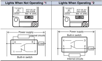
\*1. The lamp is lit when the actuator is at the free position. The lamp will be off when the contacts of the Limit Switch have been
