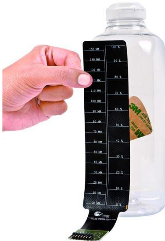
Figure 2-5. Placing the Sensor
