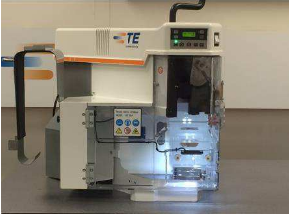
AMP-O-LECTRIC Model "G" II Terminator 2217000-[ ]
