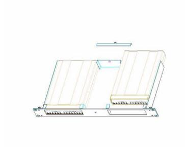
3. Mount the BA2X1U in your 19' rack using the mounting screws that match your rack's thread size. Follow the rack manufacturer's documentation to safely and securely mount the BA2X1U in the 19' rack.
