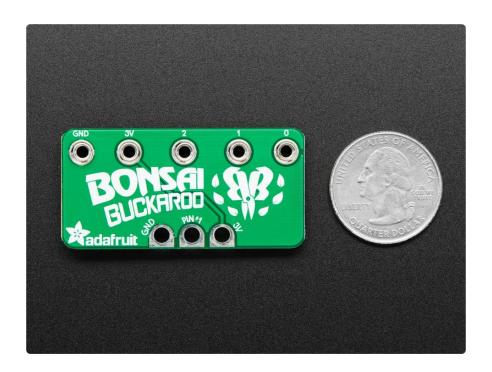
Works with micro:bit in Arduino, MicroPython or MakeCode. For CLUE, you can use CircuitPython or Arduino.
