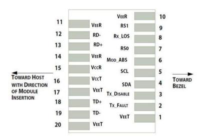
Pin-out of connector Block on Host board
