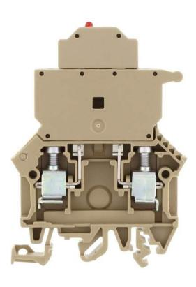
Fuse-disconnect terminal, Screw connection, Mounting type:Mounting rail TS 35/7.5 and TS 32, Rated cross-section: 10 mm², Width: 8 mm, Colour: Beige
