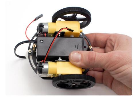
Check to see that the 9V box fits between the motors -- trim more of the inner shafts if needed.
