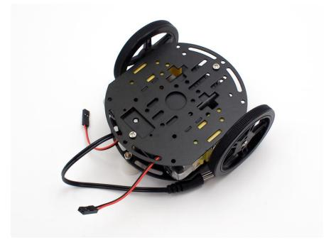
Place the middle chassis layer onto robot, making sure to fit the motor tabs into the slots of the layer, then screw in the two brass standoffs.
