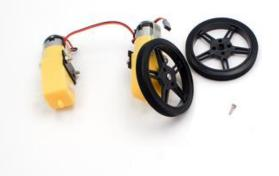
Fit the wheels onto the white knob on the motors, they will snap nicely onto the oval center.
