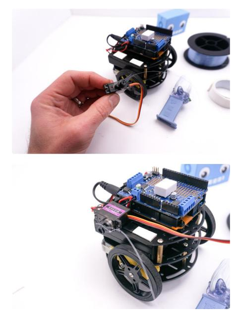
Tie the filament to the dispenser's head so the line is taut when the servo is at its resting position and when rotated downward, as seen in the images.
