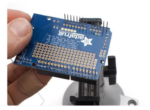
Once the headers are soldered in place, place the shield onto the Arduino 101.
