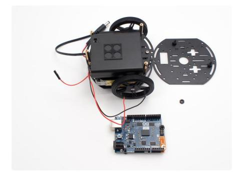
Screw in the two screws and four nuts that'll protrude from the top of the middle chassis layer as seen below, then place the layer on top of the AA battery box.
