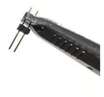
For this next step, you will need a set of pliers. First, grab the long header pins that are attached together and break them into 2 sets of 2 header pins. Then, grab them in the pliers like shown here, and then slightly bend them so they look like the next picture.
