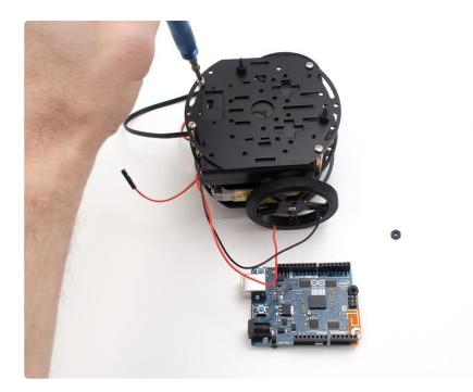
Place the Arduino 101 onto the top chassis layer, lining up the screws, then place the remaining nut onto the lower right screw to hold it in place. The upper left screw can't accommodate a nut due to the header row, but the screw will prevent the board from rotating.
