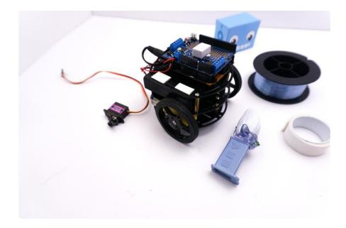
Mount the servo, tie the filament to one of the servo horn's holes.
