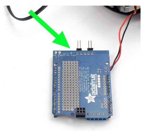
Then, solder a length of wire to the optional servo power pin (the "Opt. Servo" pin closest to the large capacitor and reset button") on the MotorShield that can be screwed into the + power terminal.
