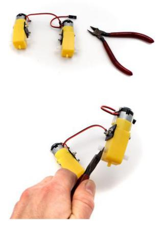
To make space for the 9V battery pack later, trim the excess off of the inner motor wheel shaft on each motor. Grab some diagonal cutters (scissors or a hobby knife will work in a pinch) and trim off about half the length of the motor wheel shaft that is on the same side as the black plate you affixed.
