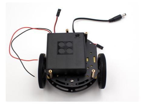
Notice the battery box is lined up on the left side of the middle chassis plate. It should be just in-between the upper left stand-off and the lower left stand-off (not touching either). This will make sure the on-off switch lines up just right in the hole of the top plate.
