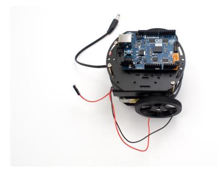
Route the wires up through the chassis layers for connecting them later to the MotorShield.
