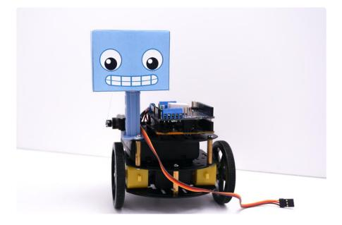
Plug the servo cable into the Servo 1 port on the MotorShield.
