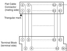
Note: All pins on the Flat Cable Connector correspond 1-to-1 to the terminal of the same number on the terminal block as shown above.
