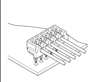
The DD and DS right angle board-in insulation displacement connectors measure just 3.5 mm in mounting height and 4.3 mm in width. Since these right angle connectors are connected to wires running parallel to the printed circuit board, electronic equipment can have a lower profile. These connectors are suited for the high density wiring of electronic products.
