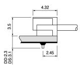
Note: 1. The above figure is the figure viewed from soldering side. 2. Tolerances are non-cumulative:  $\pm$  0.05mm for all centers.
