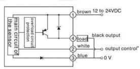
\*DARK-ON mode white ---12 to 24VDC LIGHT-ON mode --- 0V
