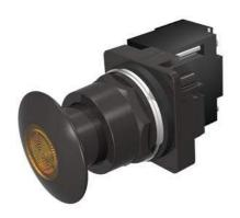
30mm BlackMax, Epoxy Coated Corrosion Resistant Complete Metal Unit Illuminated Push-Pull Operator Transformer type, 120V AC LED Lamp Mushroom Head Cap Small 1 3/4" (44.5 mm) Metal, Black with Amber Lens 3 Position Pull-Momentary/Push-Maintained UL Listed, CSA Certified NEMA 1,3,3R,4,4X,12,13 & Automotive Standards
