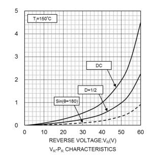
REVERSE POWER DISSIPATION:P<sub>R</sub>(W)
