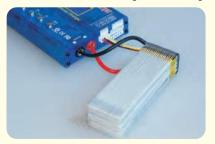
The main battery leads must be connected along with the balance lead connector as shown before charging your battery  $\dots$
