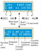
Charging current will become lower when it progress to the end of charging. Aspecific CV process will be reduced to end the charging process earlier. In fact, the charging current will goes to 1/5 when the charging process comes to 1/10. Charging capacity will be a little smaller than normal charging, but charging time will be shortened accordingly.
