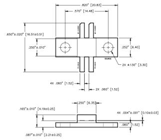
UNLESS OTHERWISE NOTED, TOLERANCES ARE INCHES  $\pm .005"$  [MILLIMETERS  $\pm 0.13$ mm]
