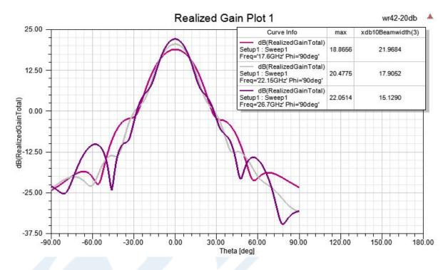
WR-42 Standard Gain Horn with 20 dBi gain, 2.92mm Female connector from Pasternack Enterprises has same day shipment for domestic and International orders. Our RF, microwave and millimeter wave products maintain a 99.4% availability and are part of the broadest selection in the industry.
