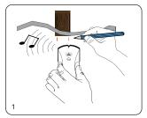
Using an edge-to-edge stud finder, find the edges of the stud.
