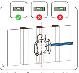
Using the wall mount as a template, mark four holes for drilling on the centerline of the stud.
