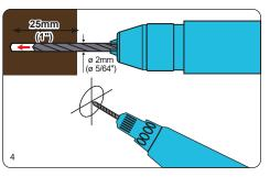
Using a power drill and 5/64" drill bit, drill pilot holes of 5/64" (2mm) diameter and at least 1" (25 mm) depth.
