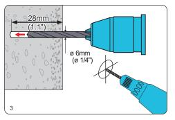
Using a power drill and 1/4" drill bit, drill pilot holes of 1/4" (6mm) diameter and at least 1.1" (28 mm) depth.
