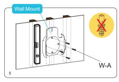
Using a Phillips screwdriver, mount the wall mount and fasten with the provided screws (W-A).
