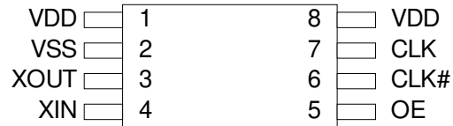
Figure 1. 8-pin TSSOP pinout
