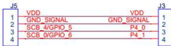
Figure 4-6. UART Connection to PSoC 4
