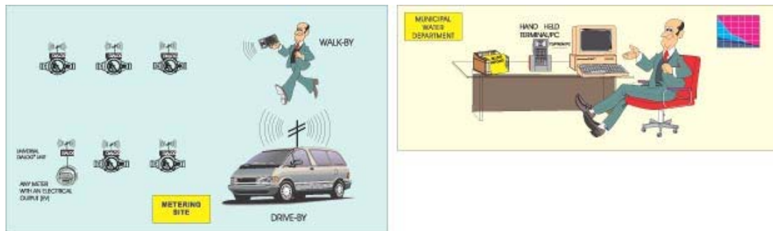
Figure 6–5. Overview of the AMR System
