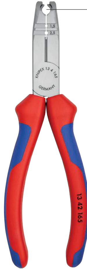
Circular cutting edge with depth limit: for easy dismantling without damaging the conductor insulation
