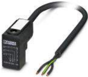
Sensor/Actuator cable, 3-position, PVC, Black RAL 9005, Free cable end, on CI valve plug (9.4 mm), Cable length: 5 m
