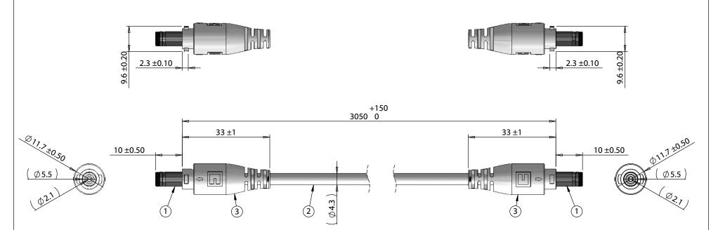
Plugs mate with cable assembly: 10-02935 & 10-02979 Functionally equivalent components may be substituted
