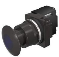
30mm BlackMax, Epoxy Coated Corrosion Resistant Complete Metal Unit Illuminated Push-Pull Operator Transformer type, 120V AC LED Lamp Mushroom Head Cap Small 1 3/4" (44.5 mm) Metal, Black with Blue Lens 3 Position Pull-Momentary/Push-Maintained UL Listed, CSA Certified NEMA 1,3,3R,4,4X,12,13 & Automotive Standards
