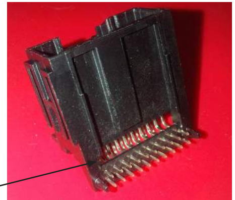
Underside view of header showing Pin-Alignment-Plate
