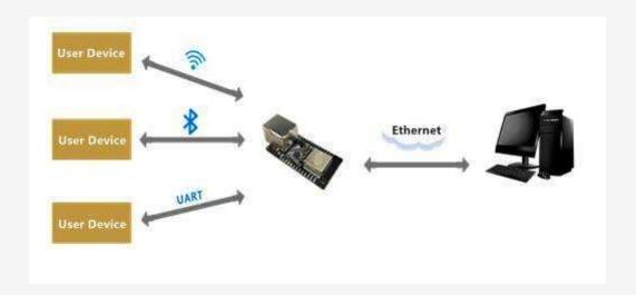
The module can be used in agriculture, industry, medical equipment, and other fields. It is an excellent choice for data transmission in IoT scenarios, such as smart agricultural sensor data monitoring.
