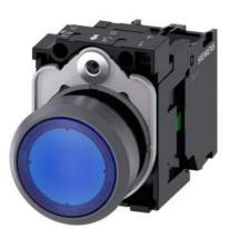
Illuminated pushbutton, 22 mm, round, plastic with metal front ring, blue, pushbutton, flat, momentary contact type, with holder, 1 NO, LED module with integrated LED 110 V AC, screw terminal
