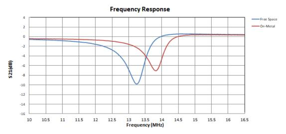
\*HF sensitivity shown in the figure is measured by Testram T8200UD Loop Antenna 10phi. Actual sensitivity performance is subject to the environment in practice.
