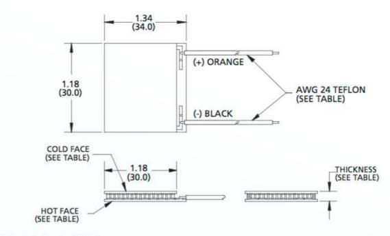
Ceramic Material: Alumina (Al<sub>2</sub>O<sub>3</sub>) Solder Construction: 271°C, Proprietary
