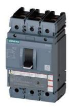
circuit breaker 3VA5 UL frame 250 breaking capacity class C 100kA @ 480 V 3-pole, line protection TM230, FTAM, In=225A overload protection Ir=225A fixed short-circuit protection li=5...10 x In UL489 SB (naval), 50 deg. cel. nut keeper kit on both sides
