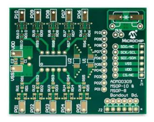
The MSOP-10 and MSOP-8 Evaluation Board is a bond-out board that allows the system designer to quickly evaluate the operation of Microchip Technology's devices in any of the following packages:
