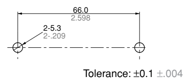
Mounting hole pattern (TOP VIEW)
