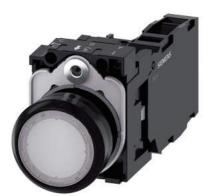
Illuminated pushbutton, 22 mm, round, plastic, white, pushbutton, flat, momentary contact type, with holder, 1 NO+1 NC, LED module with integrated LED 230 V AC, screw terminal
