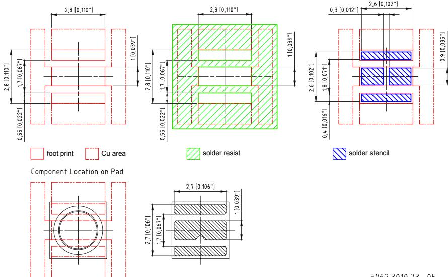
For superior solder joint connectivity results we recommend soldering under standard nitrogen atmosphere. Further information can be found in our Application Note: "Handling and Processing Details for Ceramic LEDs".
