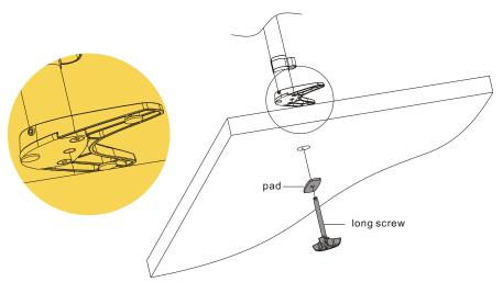
Insert the long screw into the base plate through the hole and pad (P-D) as shown above. Then tighten the long screw to hold the mount securely.
