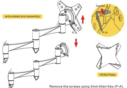
Remove the screws using 3mm Allen Key (P-A). Lift and detach the VESA plates from the mount.
