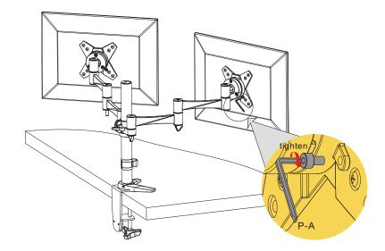
Attach the VESA plates to the mount with the retained screws from Step #2 (see page 3) and tighten them using a 3mm Allen Key (P-A).
