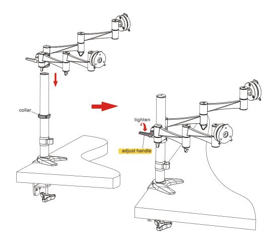
Insert the articulated arm assembly into the pole until it touches the collar. Then tighten the adjust handle.
