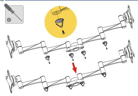
Install cable clips with the provided screws using a Philips screwdriver.
