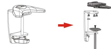
Disassemble the desk clamp and select the right parts for using grommet installation.
