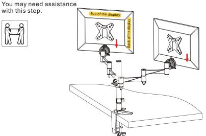
Lift your display and guide the screws into the mounting holes on the mount
