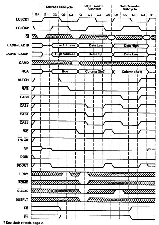
Figure 8. Dynamic Bus Sizing, Write-Cycle Timing
