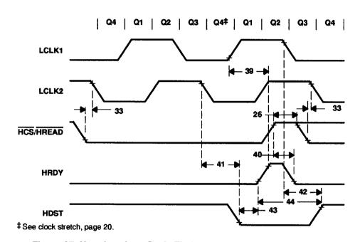
Figure 37. Host-Interface-Cycle Timing Responses (Random Read Cycle)
