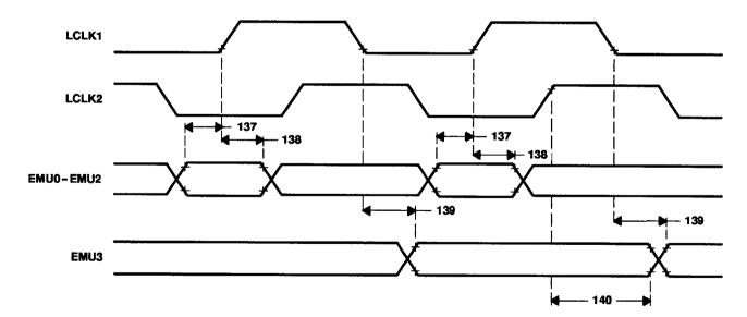
Figure 51. Emulator-Interface Timing
