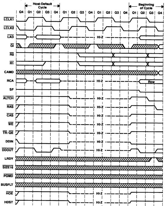
Figure 18. Multiprocessor-Interface-Cycle Timing (High-Impedance Signals)
