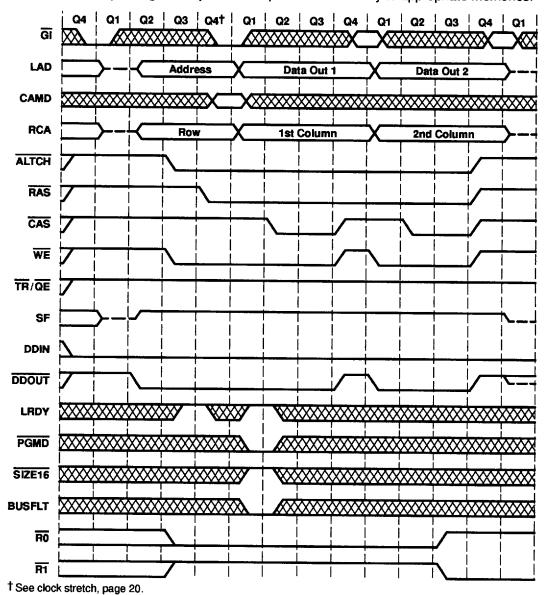
Figure 12. Block-Write-Cycle Timing (With Mask)
