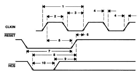
Figure 33. CLKIN and RESET Timing Requirements
