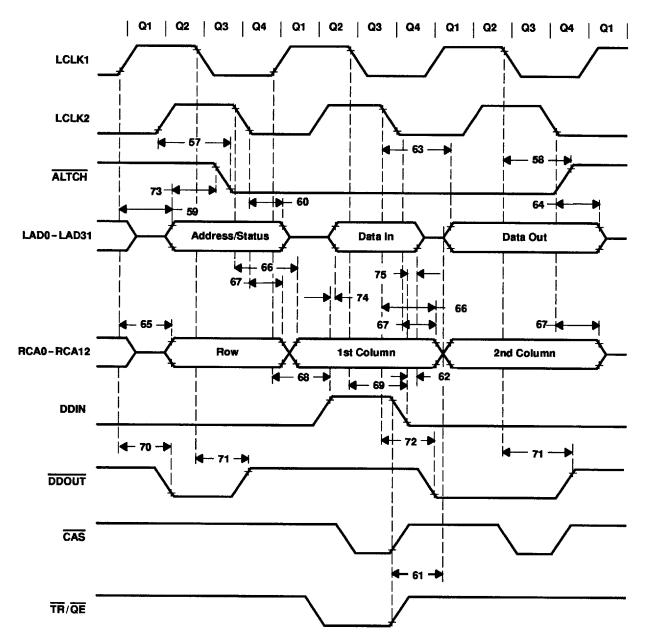
Figure 41. Local-Bus Timing: Bus Control Inputs (Continued)
