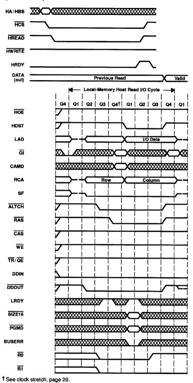
Figure 22. Host-Read Cycle Timing From SMJ34020A I/O Registers
