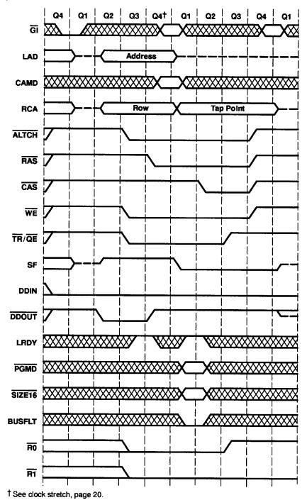
Figure 17. Serial-Data-Register-to-Memory Cycle Timing (VRAM-Alternate-Write Transfer)
