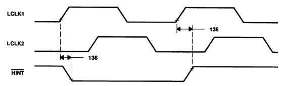
Figure 50. Host-Interrupt Timing: HINT
