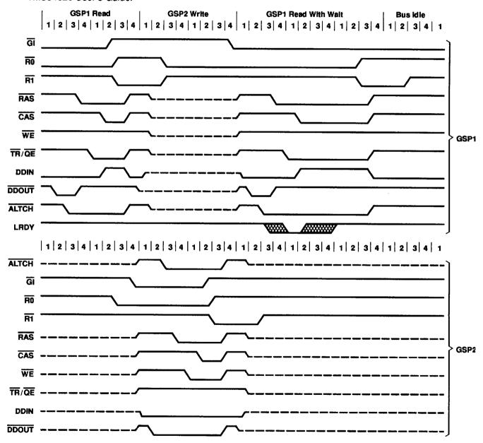
Figure 19. Multiprocessor-Interface Cycle Timing (Passing Control)
