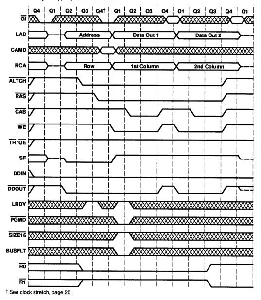
Figure 11. Block-Write-Cycle Timing (Without Mask)
