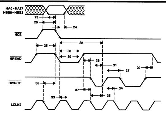
Figure 36. Host-Interface-Cycle Timing Requirements
