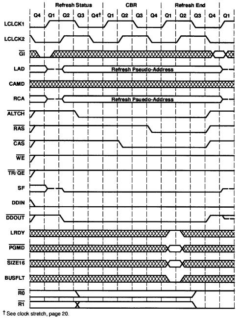
Figure 6. Refresh-Cycle Timing
