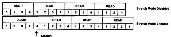
The stretched cycles are designed to accommodate worst-case 32-bit page-mode accesses, so during some nonpage-mode memory accesses stretches that are not essential can be generated. For example:
