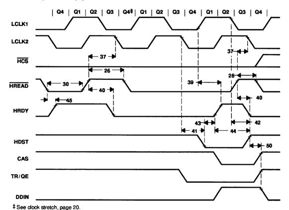
Figure 38. Host-Interface-Cycle Timing (Block-Read Cycle)
