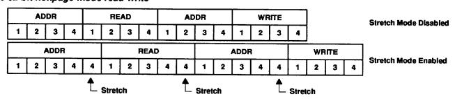
Stretches are inserted in read-modify-write accesses to help ease bus turn-around timings. In the above example, the second stretch is not needed to help these timings because the read/write turn-around has the whole of the address cycle to evaluate.
