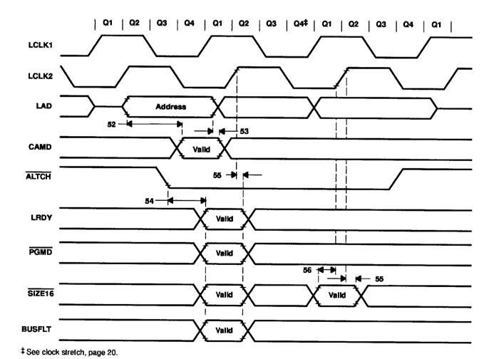
Figure 40. Local-Bus Timing: Bus Control Inputs
