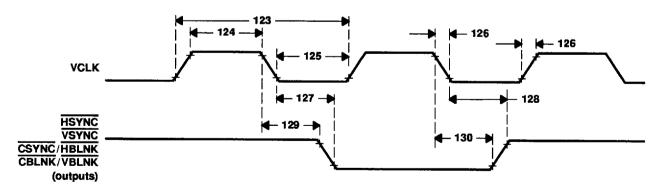
Figure 47. Video-Interface Timing: VCLK and Video Outputs
