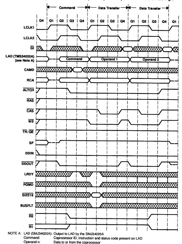
Figure 25. Transfer SMJ34020A Register(s) to Coprocessor (One or Two 32-Bit Values)
