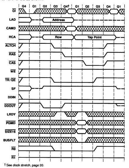
Figure 15. Memory-to-Split-Serial-Data-Register-Cycle Timing (VRAM Split-Register Read Transfer)
