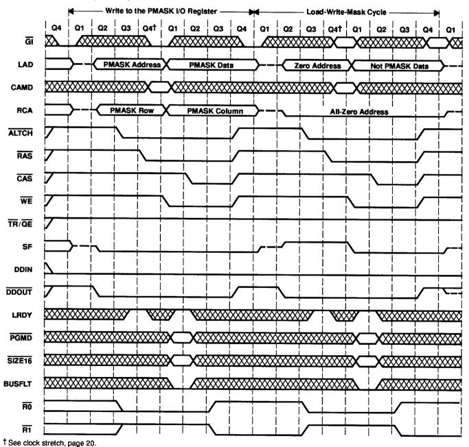
Figure 9. Load-Write-Mask-Cycle Timing
