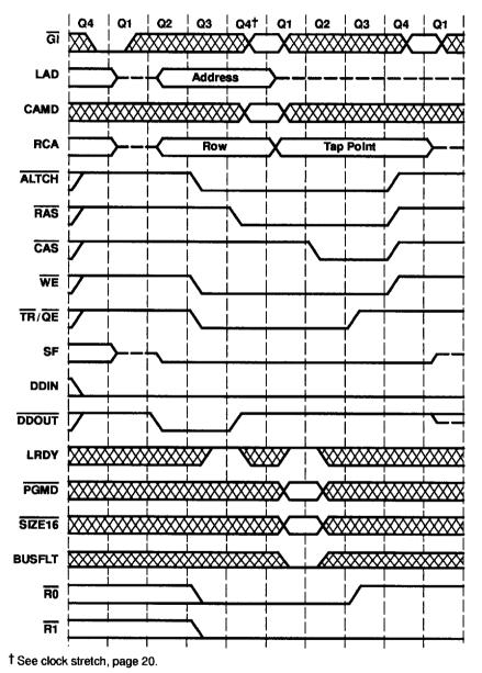
Figure 16. Serial-Data-Register-to-Memory-Cycle Timing (VRAM-Write Transfer, Pseudo-Write Transfer)
