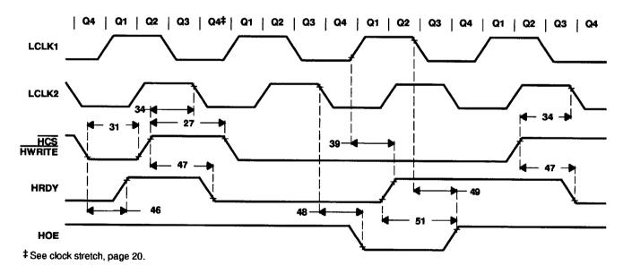
Figure 39. Host-Interface-Cycle Timing Responses (Write-Cycle)
