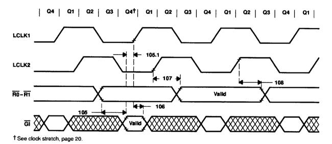
Figure 44. Multiprocessor-Interface Timing: GI, ALTCH, RAS, RO and R1
