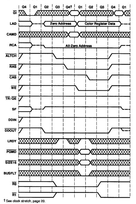
Figure 10. Load-Color-Latch-Cycle Timing
