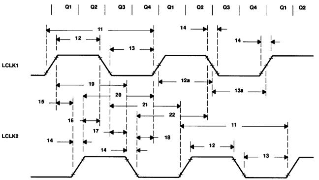
NOTE A: Although LCLK1 and LCLK2 are derived from CLKIN, no timing relationship between CLKIN and the local clocks is to be assumed, except the period of the local clocks is four times the period of CLKIN.
