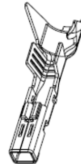
Receptacle Terminal (Sealed)
