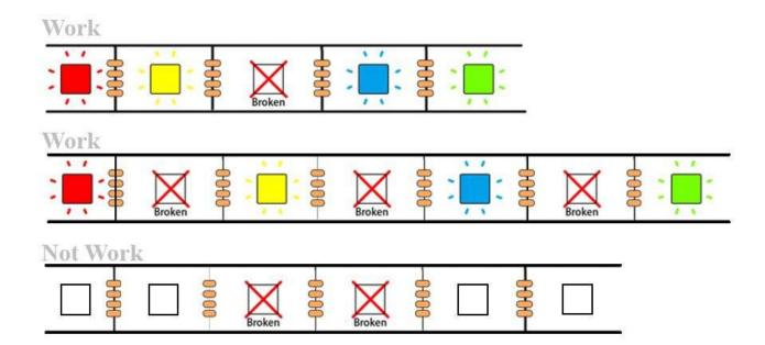
As long as not two or more adjacent LEDs are broken, the remaining LEDs will be able to work normally
